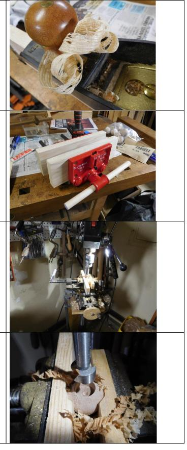
Remember that ball #2 needs a pilot hole for the screw. To center it perfectly, I kept the setup exactly as it was and just changed the drill bit. Note the sacrificial wooden bottom scrap. It is necessary to keep the drill bit from bottoming out on the metal vise.
