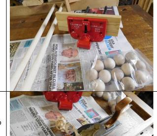
Here is the nice hickory stock that I am using for the jaw inserts. The first order of business to to joint the edge and make it smooth and flat. This operation is easier to do before the jaws are cut to length. Here is a close up shot of the Lie Nielsen low angle plane in action. Check out those thin shavings.
