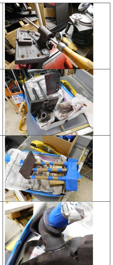
A good woodworker has a good scrap bin and I am no exception. I found a long cutoff, sawed it in half, wrapped it in newspaper and used it to both cover the static face bearings and also help mounting. I covered the leadscrew hole with a circular piece of tape. More scraps were used to make a stand for the rear face.
