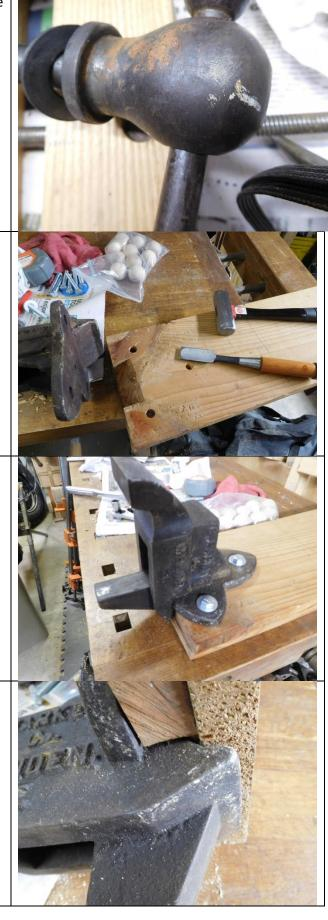
Unfortunately, the perfection does not apply to the vise mounting. It is common construction on vises of this era to have a leadscrew nut which sits in a dovetail. I removed this nut to clean it and also to clean the female dovetail slot. Here is the nut and the bent pin which holds it in place.
