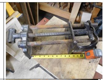
Woodworking vises generally have a cotter pin on one of the guide rods which is used as a stop. Once the vise is fully extended and the guide rod meets the end of the static face bearing, this pin prevents further extension. Of course, removing the pin allows disassembly of the vise. The nut housing is made like a "T". The cross piece rides on the guide bars for stability and also to prevent circular motion.
