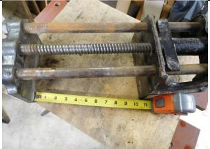
Here are the faces and the dog. Notice the odd bolts used to attach the faces. Our previous owner used suitable wood, oak, and trimmed the pieces accurately. But then he used bolts for attachment. My guess is that he was a novice woodworker who was tasked with making these jaws.
